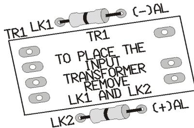
**2** Place the input transformer, keeping in mind the position of their pins (four to the left and three to the right), and solder it to the main board.
