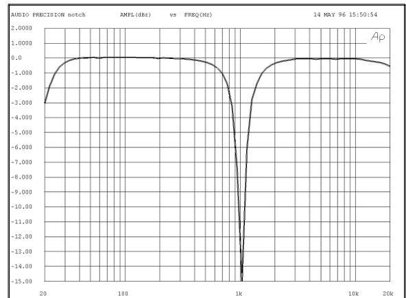
You could also make a notch filter type, selecting the highest Q (15) that the equaliser card allows. The right picture shows a notch filter type with 15 dB of attenuation at 1 kHz:
