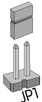
Each input has its own jumper. In the following chart is shown the correspondence between the inputs and their jumpers. This jumper is factory set to the closed position (pin 1 connected to ground).
