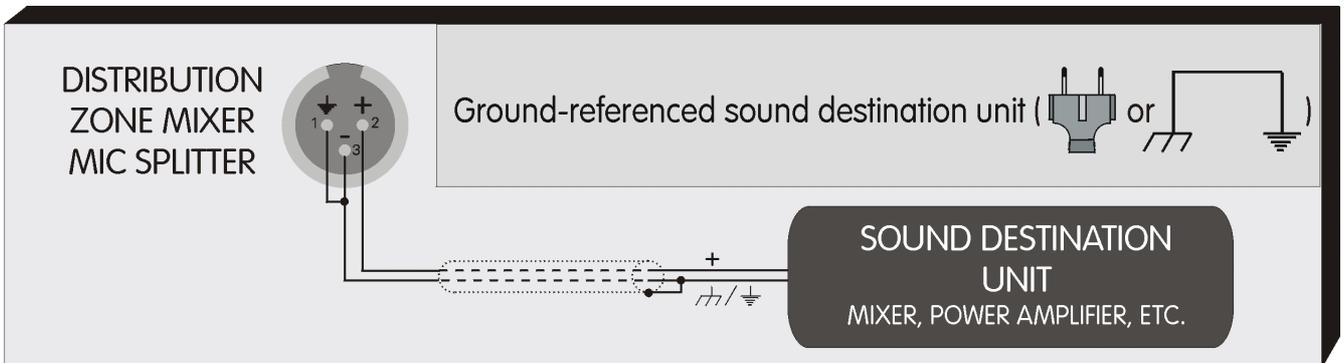
2) Using single conductor shielded cable:
