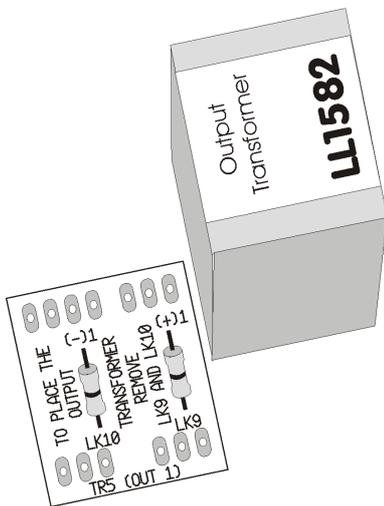
**1** Remove the links corresponding to the output transformer. In this case LK9 and LK10.
